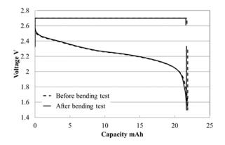
$\label{eq:charge:CV / 2.7V / cutoff 0.2C / 25 °C} Charge: CC / 2.0C / cutoff 1.5V / 25 °C$
