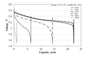
Discharge : CC / 2.0C / cutoff 1.5V /  $-40^{\circ}$ C,  $-20^{\circ}$ C,  $0^{\circ}$ C,  $25^{\circ}$ C,  $45^{\circ}$ C,  $70^{\circ}$ C
