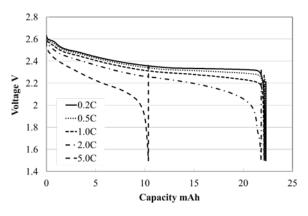
Discharge : CC / 0.2C, 0.5C, 1.0C, 2.0C, 5.0C / cutoff 1.5V /  $25^{\circ}$ C
