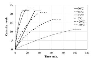
Charge : CV / 2.7V /cutoff 0.2C /  $-40^{\circ}$ C,  $-20^{\circ}$ C,  $0^{\circ}$ C,  $25^{\circ}$ C,  $45^{\circ}$ C,  $70^{\circ}$ C
