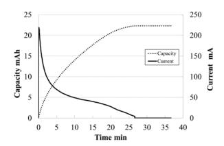
Charge : CV / 2.7V /cutoff 0.2C /  $25^{\circ}$ C
