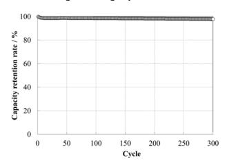
$\label{eq:charge:CV/2.7V/cutoff 0.2C / 25°C} Charge: CC / 2.0C / cutoff 1.5V / 25°C$
