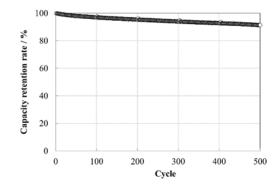
$\label{eq:Charge:CCV/4.2V/0.5C/cutoff} Charge: CC/0.5C/0.5C/cutoff C.05C/25^{\circ}C$  Discharge: CC/0.5C/cutoff C.0V/25^{\circ}C
