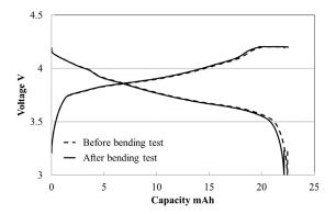
$\label{eq:CCCV} Charge: CCCV \ / \ 4.2V \ / \ 0.5C \ / \ cutoff \ 0.05C \ / \ 25^\circ C$  Discharge: CC \ / \ 0.5C \ / \ cutoff \ 3.0V \ / \ 25^\circ C
